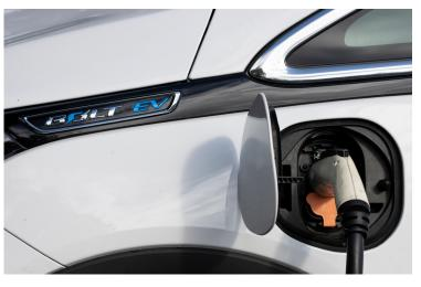
about 180 miles of range over an eight-hour charging period. A licensed electrician must install a Level 2 charger.
