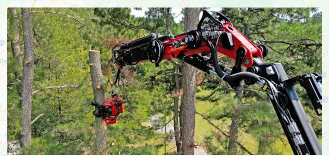
Robotic Grapple Saw safely removes trees in hard-to-reach places.
